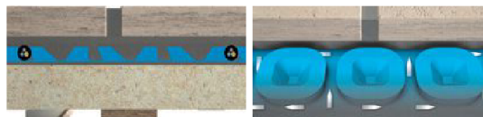
UNCOUPLING / CRACK ISOLATION
