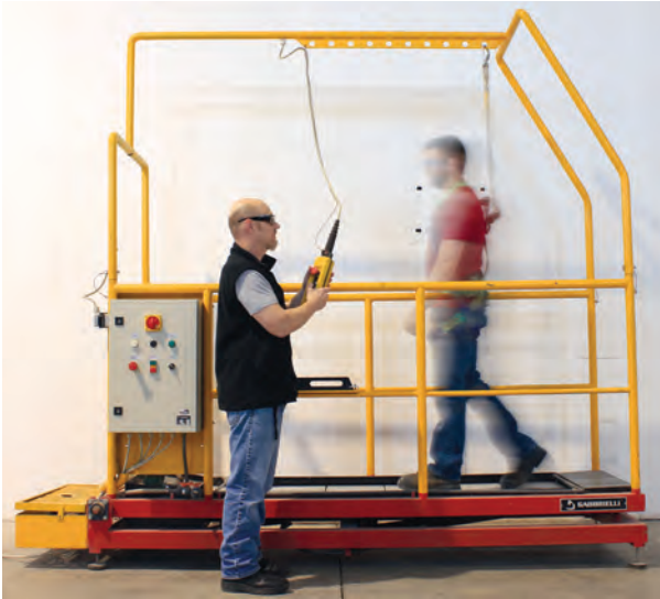
A German Ramp, similar to the one depicted above, is used in DIN 51130, and in much of the foundational research of Dr. Jens Sebald which underlies the ANSI A137.1 standard. The ramp shown is currently being used for research in the TCNA Laboratory.
