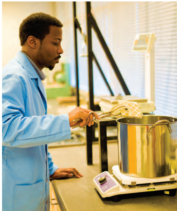
A TCNA lab technician performs the water absorption test per ASTM C373.
