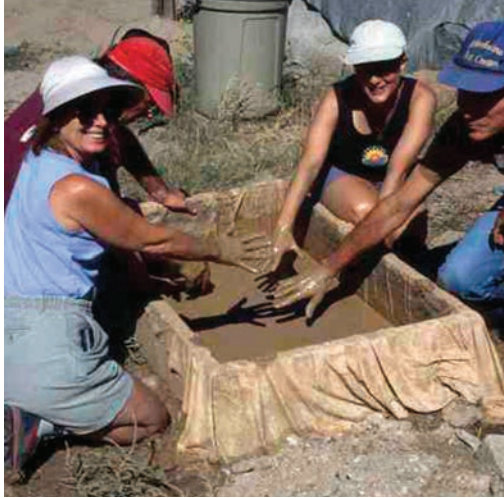
Screening raw clay dug from the mountains near La Madera, New Mexico to make tiles from scratch, a 2-day workshop at “Spirit in Clay,” in the fall of 2000.
