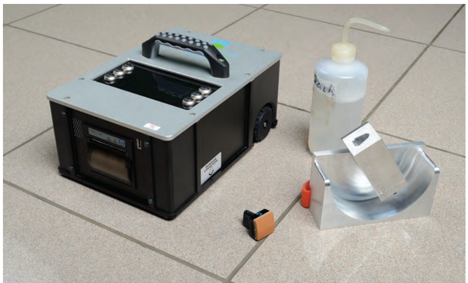
The BOT 3000E, shown here, is used for ANSI A137.1, Section 9.6, DCOF testing.
