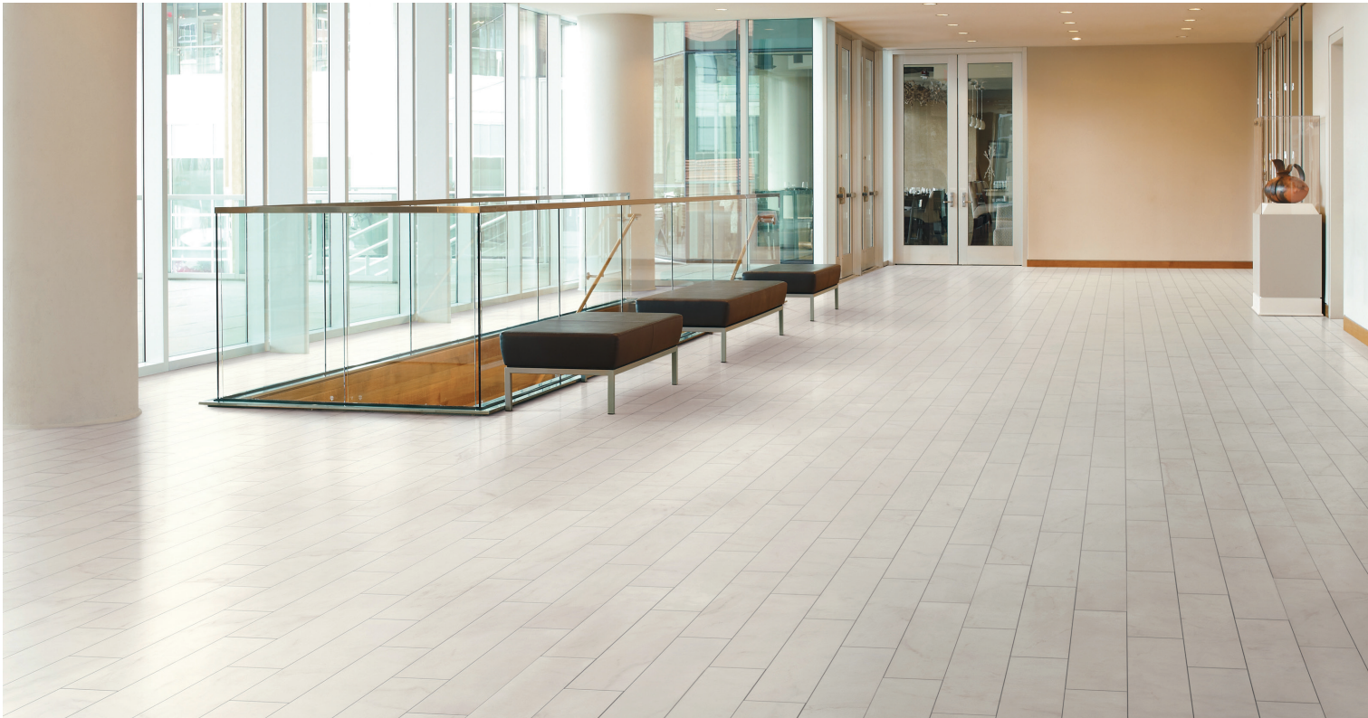
The high light reflectance value (LRV) of light-colored tiles helps maximize the efficiency of interior lighting.
