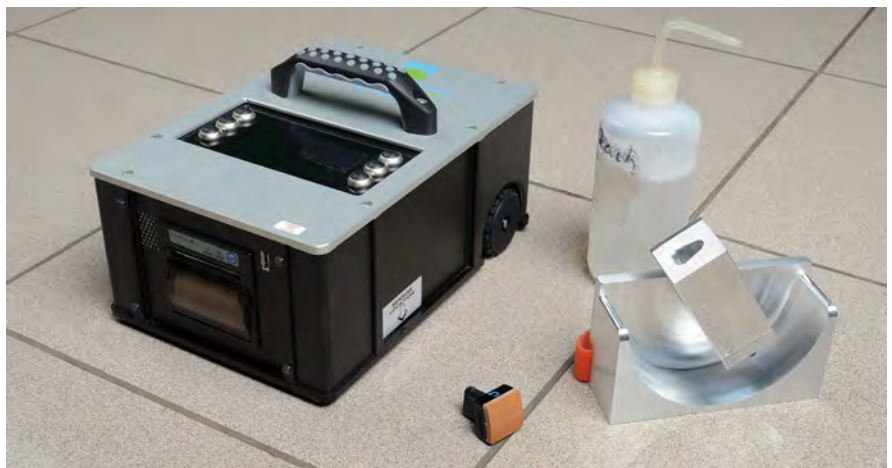
The BOT 3000E, shown here, is used for ANSI A137.1, Section 9.6, DCOF testing.
